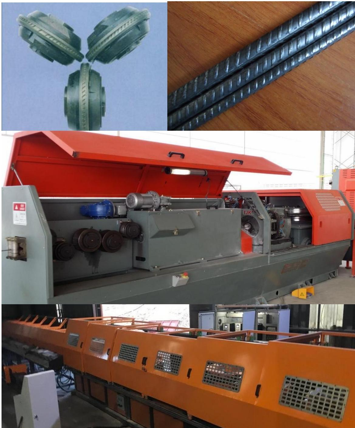
In many developing countries cold forming of rebars is a convenient and cost effective solution. Wire rods of relevant diameters are rolled under rolling cassettes to create the ribs under normal temperature. LLC "Atroy Sunny Engineering" has one of the best solutions for this project providing accurate and fast production of rebars with very reliable and long lasting equipment.
