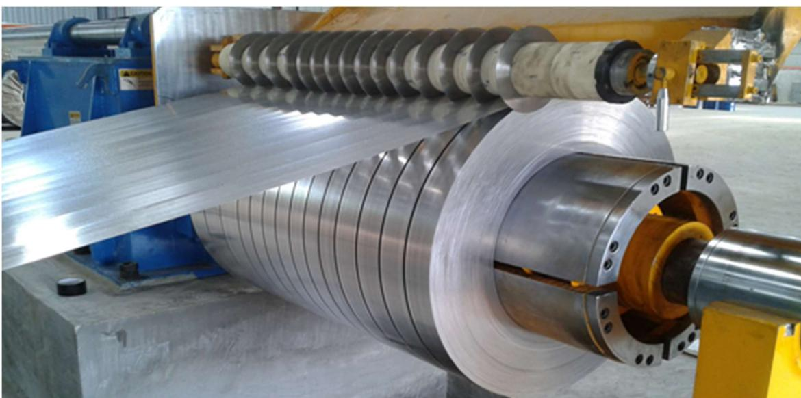
Slitting Lines are essential for Service centres and manufacturers of Pipes, Angles, Channels, Purlins and Profiles. We can provide specialised slitting lines for all applications for low carbon steel, high carbon and stainless steel, aluminium coils and plates. We offer slitting lines up to 10mm thickness and width up to 2000mm and speed up to 180 meters per minute.
