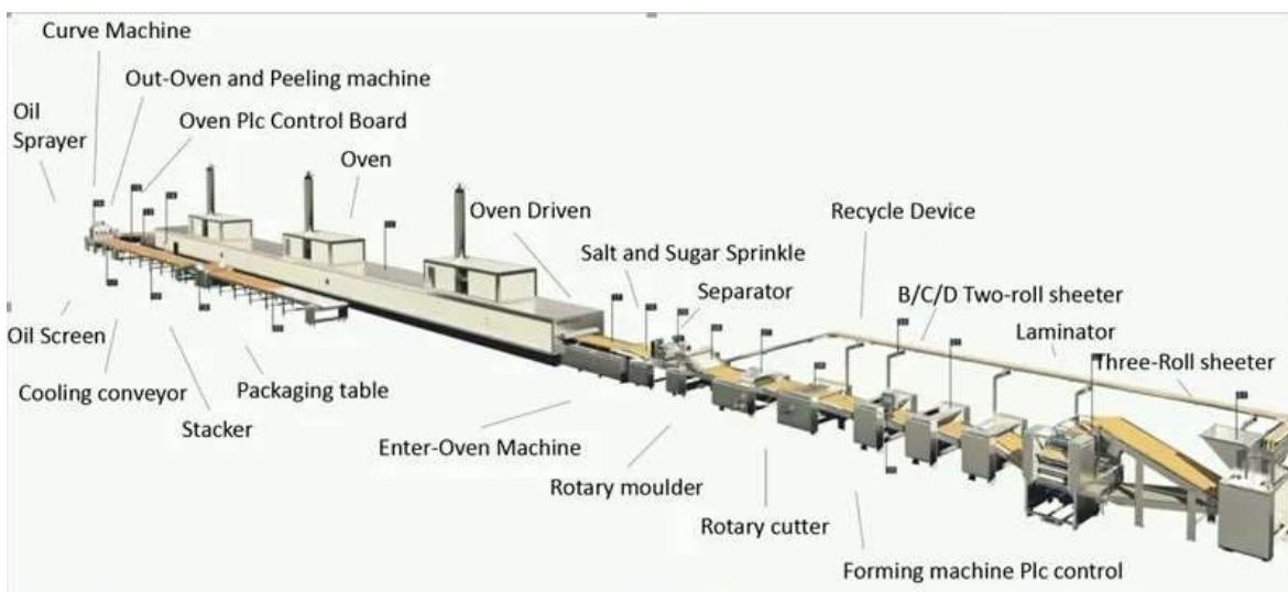
This biscuit processing machine is an advanced equipment for making various kinds of biscuit, such as crisp biscuit, cookies, sandwiching biscuit with a middle layer. LLC "Atroy Sunny Engineering" specialises in providing economical solutions for building automatic biscuit production lines suitable for developing markets.
