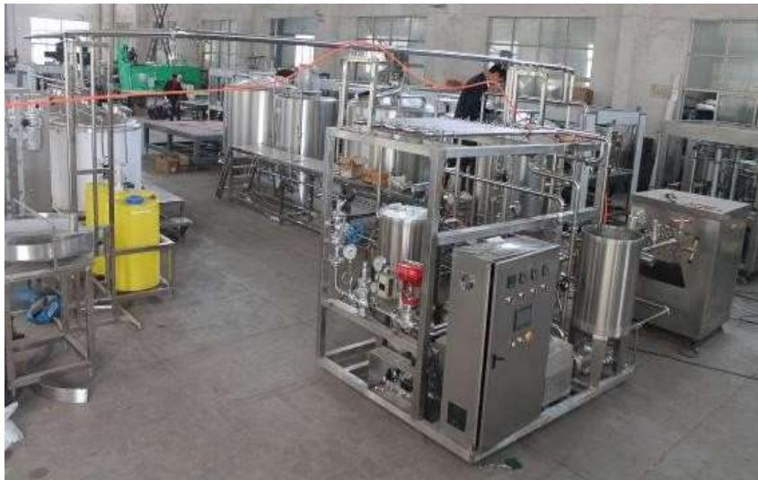
LLC "Atroy Sunny Engineering" can provide fully integrated low-cost line to produce a variety of fruit juices with superior quality and attractively packed in paper cartons. The system includes water purification unit, juice mixing unit, sterilization and packaging units and also system cleaning equipment.
